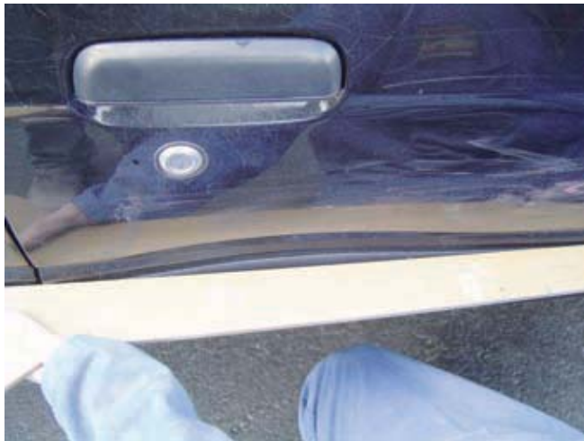
Figure 3 Close-up of damage. A straight edge is used to accentuate the damaged area
